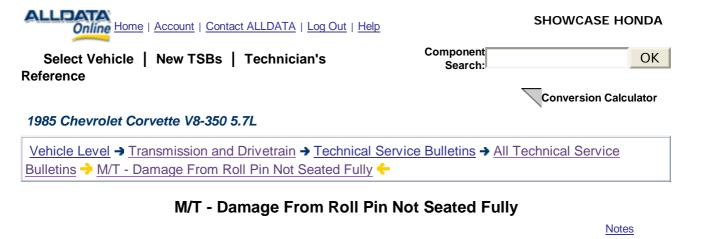
85-31 7B Feb., 1985 Subject: DAMAGE TO TRANSMISSION DUE TO IMPROPERLY INSTALLED **REVERSE IDLER SHAFT ROLL PIN - DOUG NASH MANUAL** TRANSMISSION WITH AUTOMATIC OVERDRIVE
